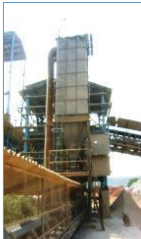
Bag filters at various material transfer points & silo top
